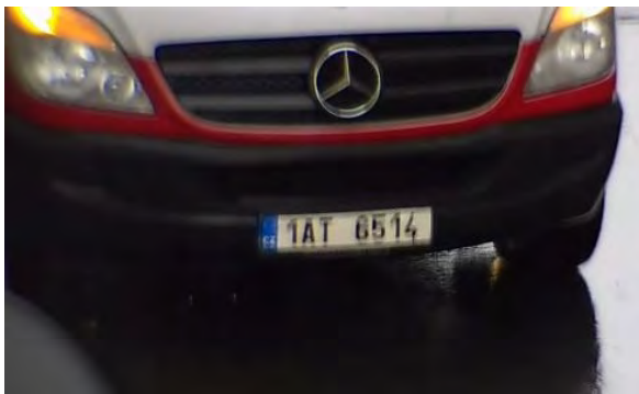
Fig. 12: Blurred license plate due to long exposure time
