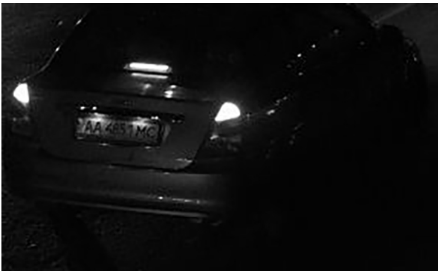
Fig. 15: Insufficient light to recognize license plate
